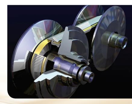
CVTs are used in new car production by Nissan, Honda, Toyota, and other manufacturers due to their smoother driving experience and increased fuel efficiency.
